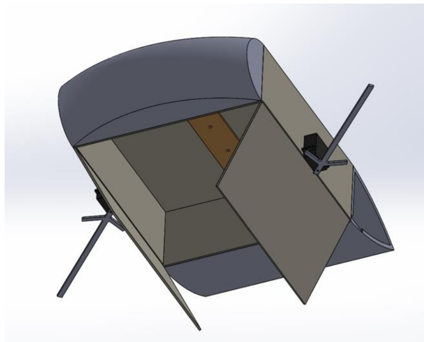
Figure 6. Final payload bay design that can hold six footballs or four water bottles.
