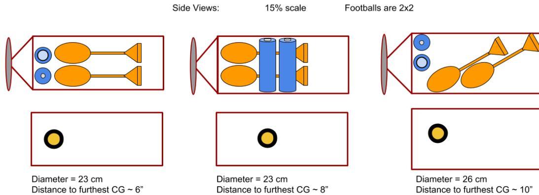
Figure 7 Payload Layout
